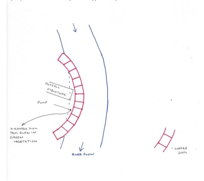
Coffer dams and diversions are to be sized to accommodate a flow of Q5, equivalent to 1.22 cumecs at the outfall site. The coffer dams shall be 1m high and will therefore be more than adequately sized. The dams shall consist of:
