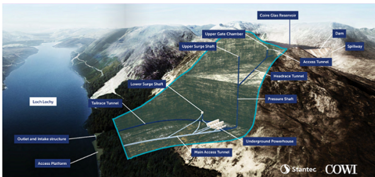
Diagram of the Coire Glas scheme showing how most of it would be underground.
