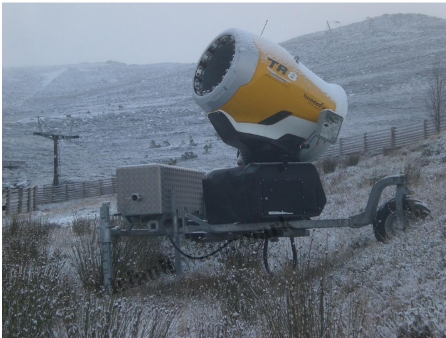
TR8 Fan Gun: There are 8 on the hill which were provided by HIE. Photo Credit: Alan Bratney
