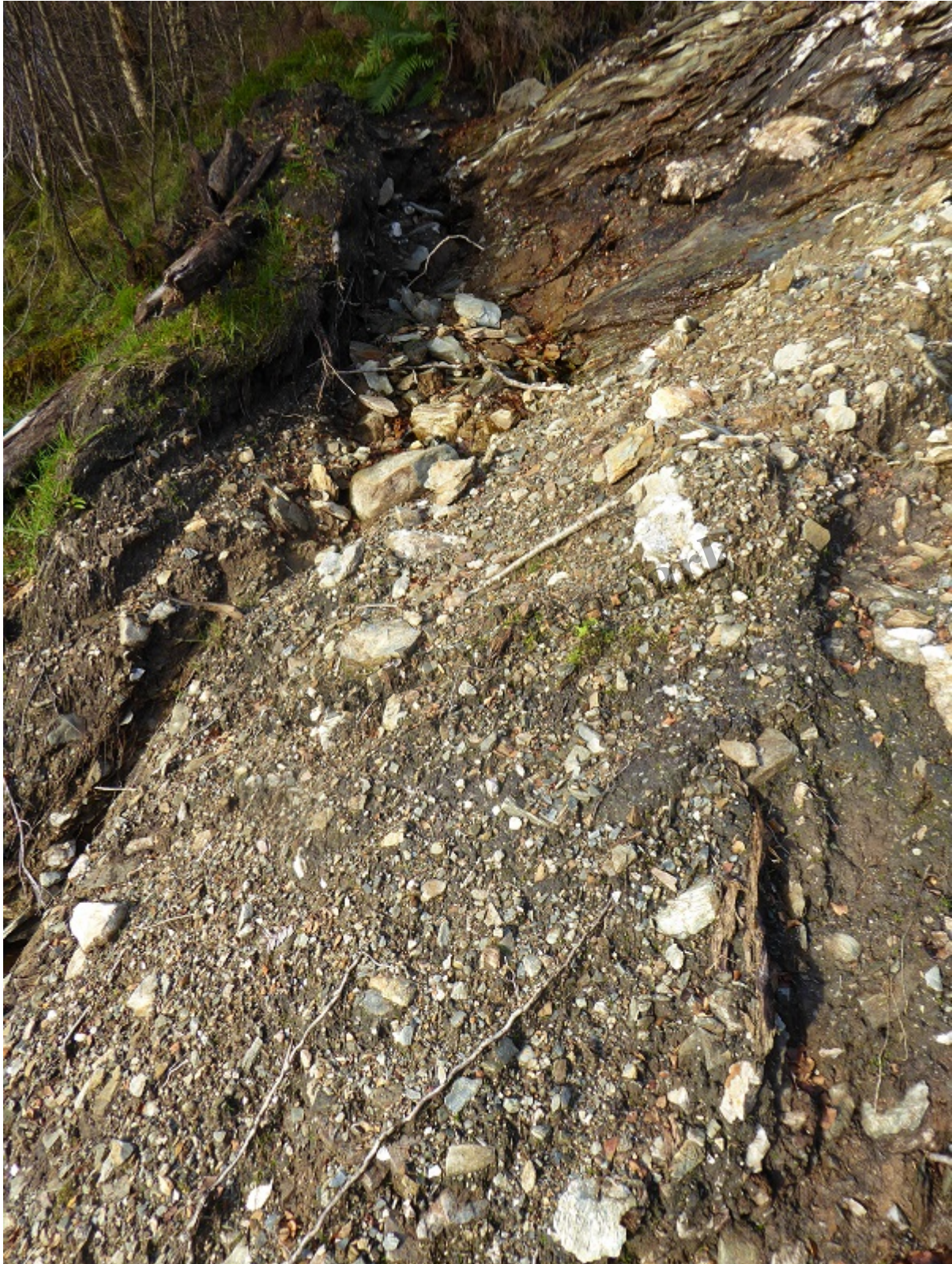
Tree roots were clearly visible on an area of soil which had remained attached to the rock slabs
