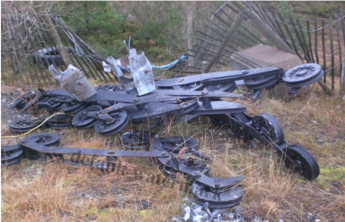
Haul rope sheaves dumped on the ground
