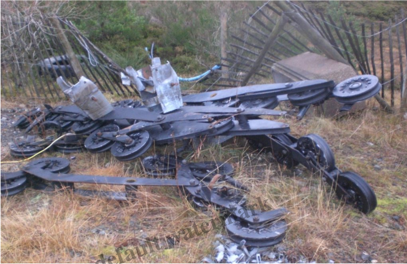
Haul rope sheaves.....dumped on the ground
