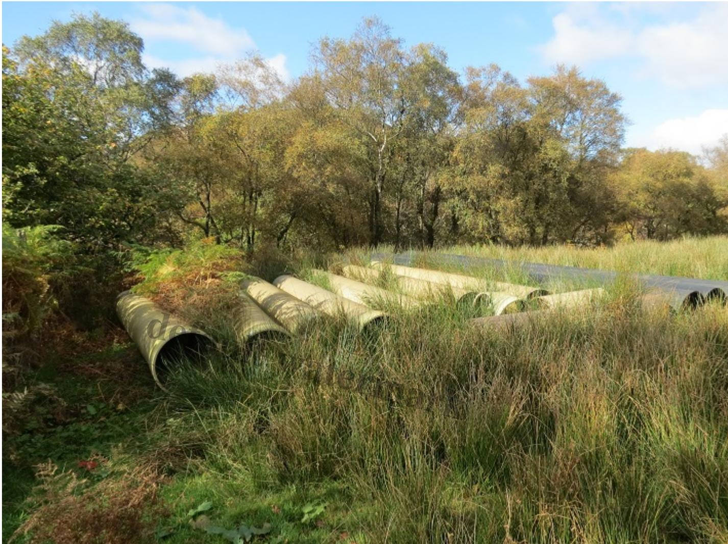
Two types of hydro pipes, glass reinforced plastic for use lower down where the water pressure is high and black for use higher up. Photo credit Louise Brimelow.
