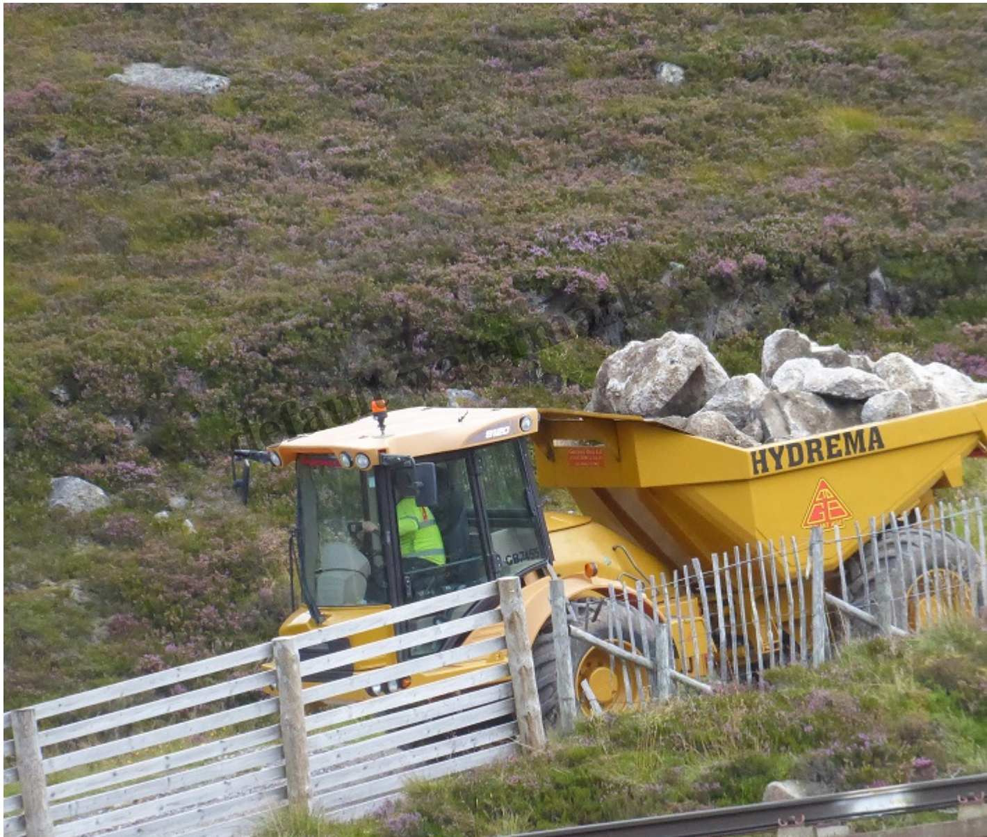
Dumper truck on hill track down from Ptarmigan carrying remains of concrete plinths from West Wall Photo Monday 28th /
